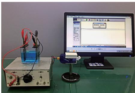
Fig 1 Device for measuring Avogadro constant by electroplating
