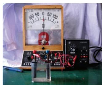
Fig 2 Conductivity of solid salt and distilled water
