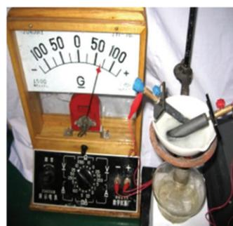
Fig 4 Conductivity of molten salt
