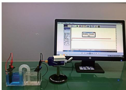
Fig 2 Device for determining Avogadro constant by dual-liquid galvanic cell method
