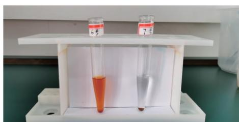
Fig 7 Test results of reaction products between acetaldehyde and new  $\text{Cu}(\text{OH})_2$  by anhydrous ethanol
